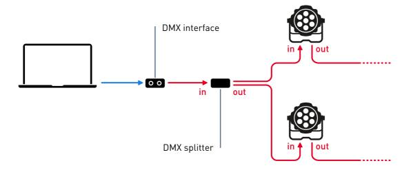
A **DMX transmitter** lets you send DMX wirelessly (shown below). Other equipment includes **DMX boosters**, which amplify the signal over long cable runs. From Lightkey's perspective it doesn't matter if you employ splitters, transmitters, boosters, or cable adapters along the DMX line. The software does not specifically control those devices and doesn't even know they're there.
