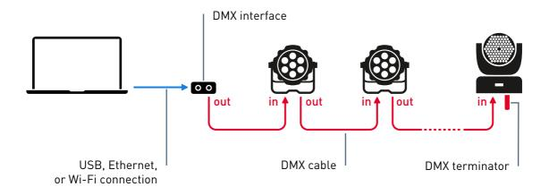
Each daisy chain of fixtures forms a **DMX universe** which operates up to 512 channels. For many installations a single universes is sufficient, but Lightkey can control up to 16 full universes or 8192 channels.
